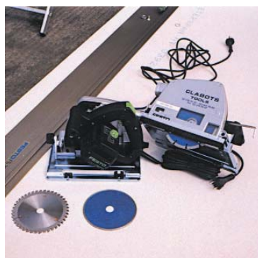
Cutting with a circular saw.
