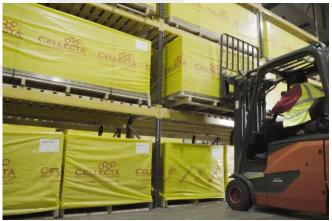
**DECKfon® 30T** is supplied on pallets, wrapped in temporary protection. This covering is to offer dust protection and is a temporary measure to protect the boards from the weather during the loading/unloading process, it is <u>not</u> a waterproof cover.
