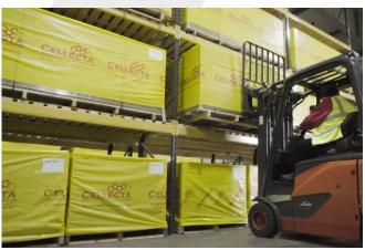
**HiDECK® Structural** is supplied on pallets, wrapped in temporary protection. This covering is to offer dust protection and a temporary measure to protect the boards from the weather during the loading/unloading process, it is **not** a waterproof cover.
