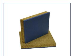
Karma Overlay 28 is a high performance acoustic floor panel with an exceptional performance to height ratio. Comprising an 18mm tongued and grooved 18mm P5 chipboard bonded to a 10mm cross linked polyolefin foam resilient layer. Karma Overlay 28 provides excellent impact and airborne sound insulation in a single product. It is used on an existing floor, new ply or chipboard floor or directly to concrete/screed floors making it an ideal product for refurbishment and new build projects.
